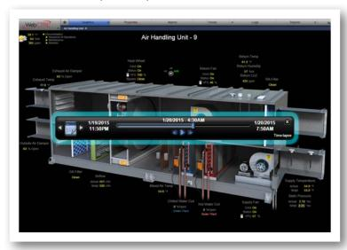
This feature allows you to roll back the clock and review real-time data on any piece of equipment connected to your Automated Logic System. This industry-leading feature is built into your existing system at no additional cost to you. Ultimately, it allows you to quickly review what happened, when it happened and why it happened without sorting through a pile of trend data. If you have never used this feature, consider trying it out.
